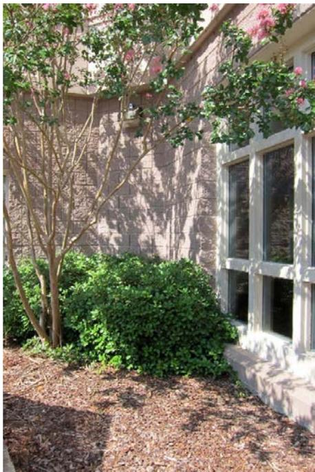
**Figure 2.** Vegetation touching the structure can provide a bridge over treated areas (Photo: Patty Alder, NCSU).
